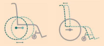
• front and rear seat-to-floor heights can be adjusted through wheel or frame adjustments or through range of different fixed-frame seat heights to optimize fit for foot propelling on folding-frame wheelchairs
