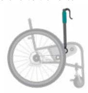
Removable trike attachment: for users of active manual wheelchairs to improve efficiency over long distances. Designed to be self-propelled by users. The attachment is removable to allow wheelchair access to small spaces such as buildings and homes. The attachment/detachment mechanism should be quick-release or removable without tools. When connected, the trike attachment lifts front castor wheels off ground when locked in place. Hand-powered drive train to front drive wheel.
