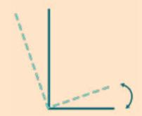
adjustable recline<sup>18</sup> with minimum 20° with tools; optional variable (adjustable without tools) recline minimum 20°
